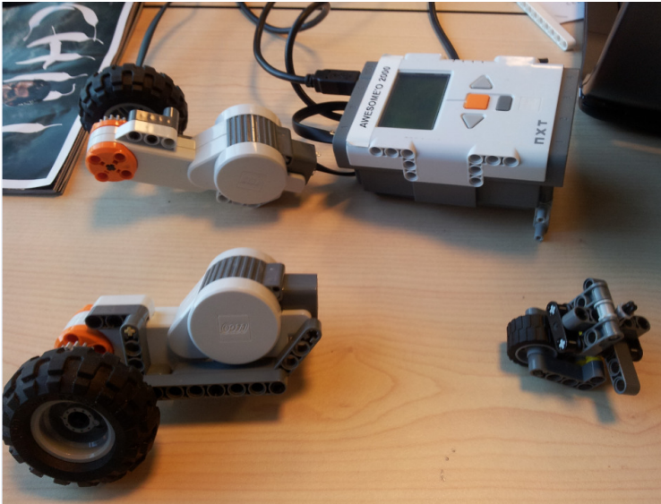
Picture 1: showing the two motors, the freewheel and the microcontroller.
