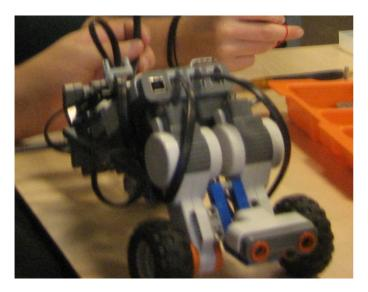
We use this robot to learn have to use the computer program, because we have used a lot of sensors on this robot. Then we connect the robot to the computer, and started try out some simple programming. We learned how to make the robot drive and stop just with a single loud pat. We were also able to make the robot start with a touch on the back of the robot.
